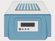
Heating block or thermomixer w/ shaker option (for heating at 56°C and shaking at 400-600 rpm) or water bath
