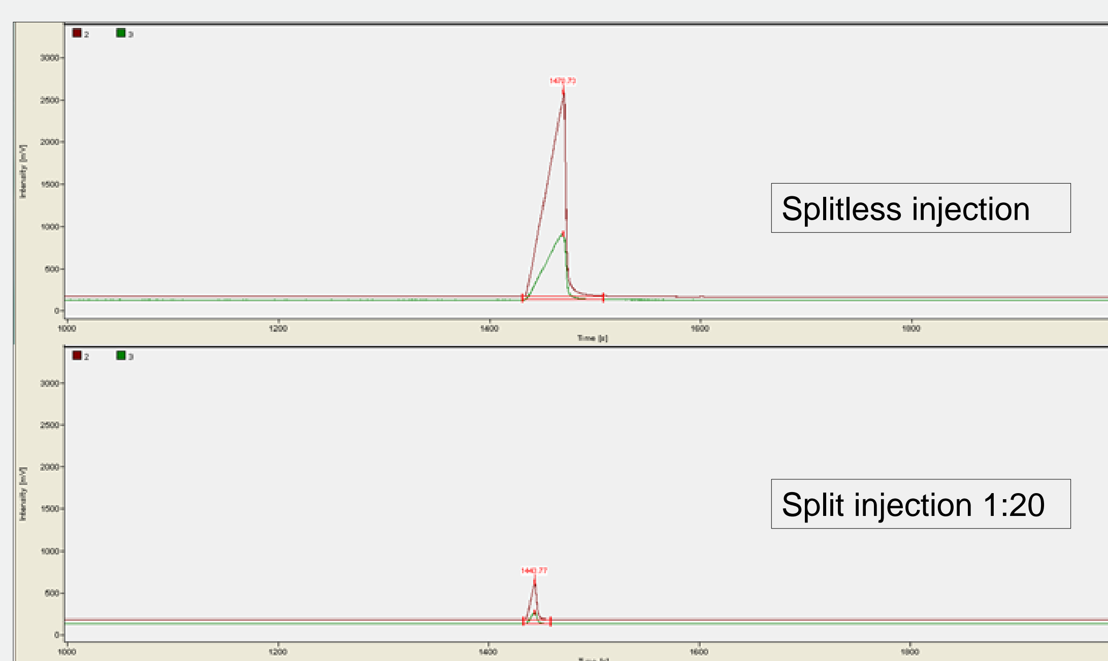
Figure 1: Standards of vanillin containing 1578ng/ \mu\text{L} analyzed using GC-P-IRMS with splitless injection (top) and split injection of 20:1 (bottom).
