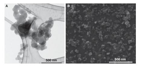
Figure 4. Printex 90 intratracheal instillation exposure characterization by TEM and SEM. (A) Transmission Electron Micrograph of agglomerated small- and medium size Printex 90 aggregates (67  $\mu$ g/mL). (B) Scanning Electron Micrograph illustrating the overall size and morphologies of Printex 90 aggregates and agglomerates in the dispersions (1.675  $\mu$ g/mL).
