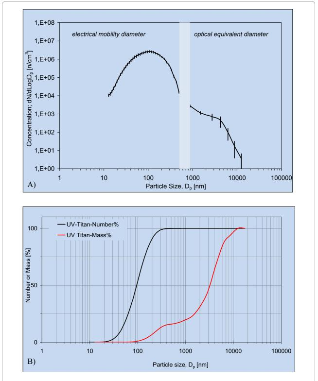
**Figure 2** Characteristics of the exposure atmosphere. A) Particle number size distribution of the UV-Titan L181 in the exposure chamber. Data are based on nine one-hour exposure measurements. Mean ± SD. B) Accumulated number and mass concentration of particle concentrations in the exposure chamber. It is assumed that the optical and mobility particle sizes can be directly compared and data gap is filled by linear interpolation.
