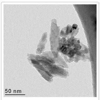
**Figure 1 TEM image of TiO**<sub>2</sub> crystallites. Transmission electron microscopy image showing the typical equidimensional to elongated morphology of the TiO<sub>2</sub> crystallites in UV-Titan L181. Bar = 50 nm.
