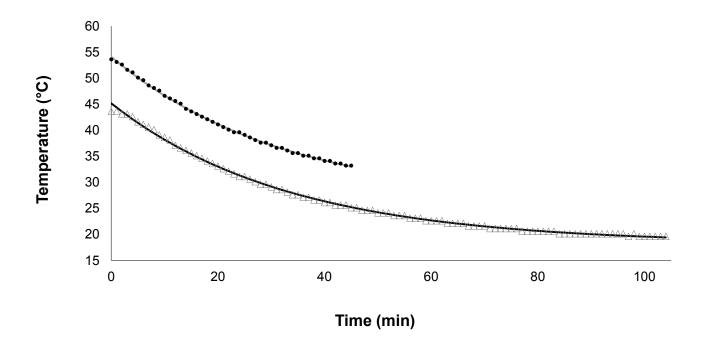
**Figure 6**. Observed ( $\bullet$ ,  $\Delta$ ) and fitted ( $\longrightarrow$ ,  $\longrightarrow$ ) temperature profiles of the cooling of meatballs in kitchens one and two, respectively. Fitting done with Newton's Law resulting in k = 1.8 min<sup>-1</sup> in both catering units.
