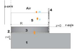
**Fig. 1.** a Part of the heating rig used for studying the contact baking process; domain 1 is the rig (aluminum block), domain 2 is the thermal conducting paste (copper paste), domain 3 is the aluminum plate (bottom part of the baking disc), domain 4 is the wall of the baking disc (stainless steel), and domain 5 is the product (pancake batter).
