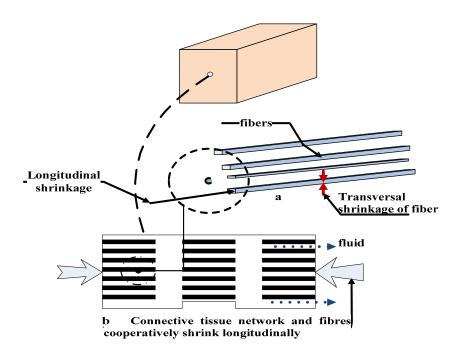
Figure 3-1 Schematic diagram of shrinkage of meat structures
