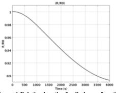
Figure 6 Relative length of cylinder as function of time (R/R0)
