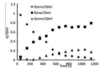
**Fig. 2b.** The extent heat used for evaporation, sensible heat and heat lose by convection to environment: (diamond = fraction of sensible heat consumed), (square = fraction of latent heat – heat used for evaporation of water), and (triangle = the fraction of heat loss to environment by convection. Notice, the latent heat was obtained from measured mass loss and the heat of evaporation; sensible heat was calculated at average product temperature using the measured temperature.
