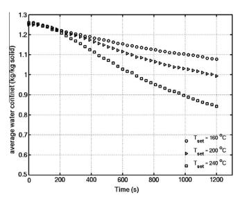
**Fig. 3.** Average water content (kg of water/kg of solid) during baking of the pancake batter at three different temperature set points (160, 200, and 240 °C, respectively). The data are only shown with a sampling interval of 30 s, for clarity.
