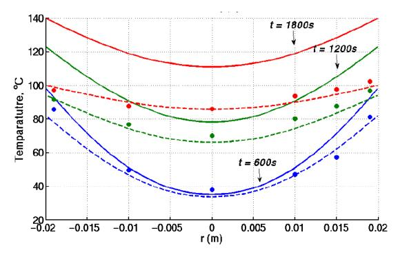
Figure 7-6 Cross sectional temperature profile of cylindrical meat, (-) pure conduction model, (--) the current model (conduction +convection + evaporation) (o) measured data
