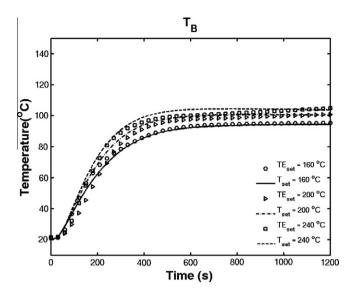
**Fig. 7.** Comparison of simulated and measured temperature profiles at position B with different temperature set point (160, 200, and 240 °C). The data are only shown with a sampling interval of 30 s, for clarity.
