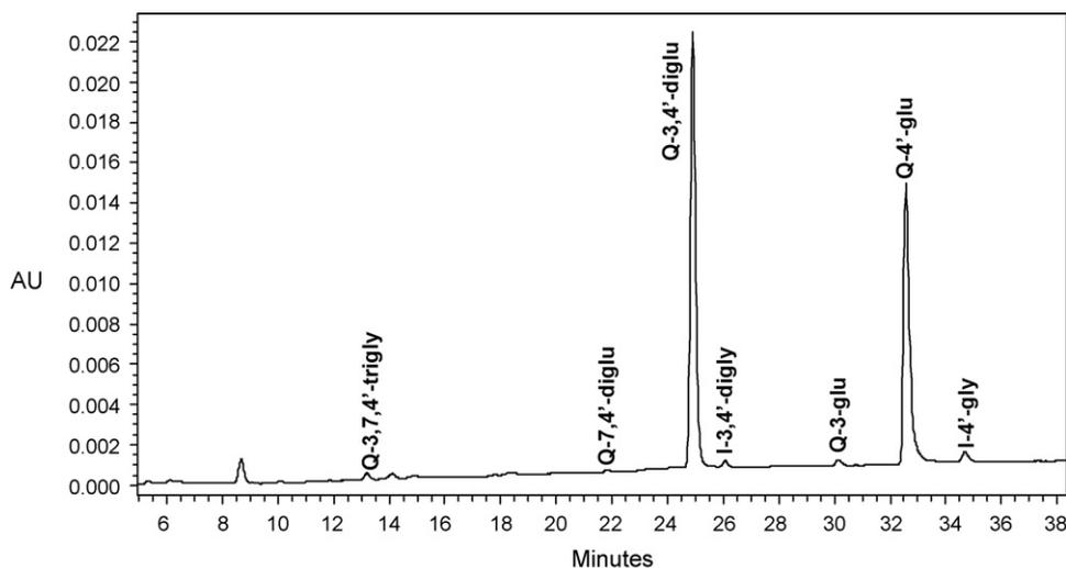
Fig. 2. Chromatogram of an onion extract (HPLC–UV, 254 nm).
