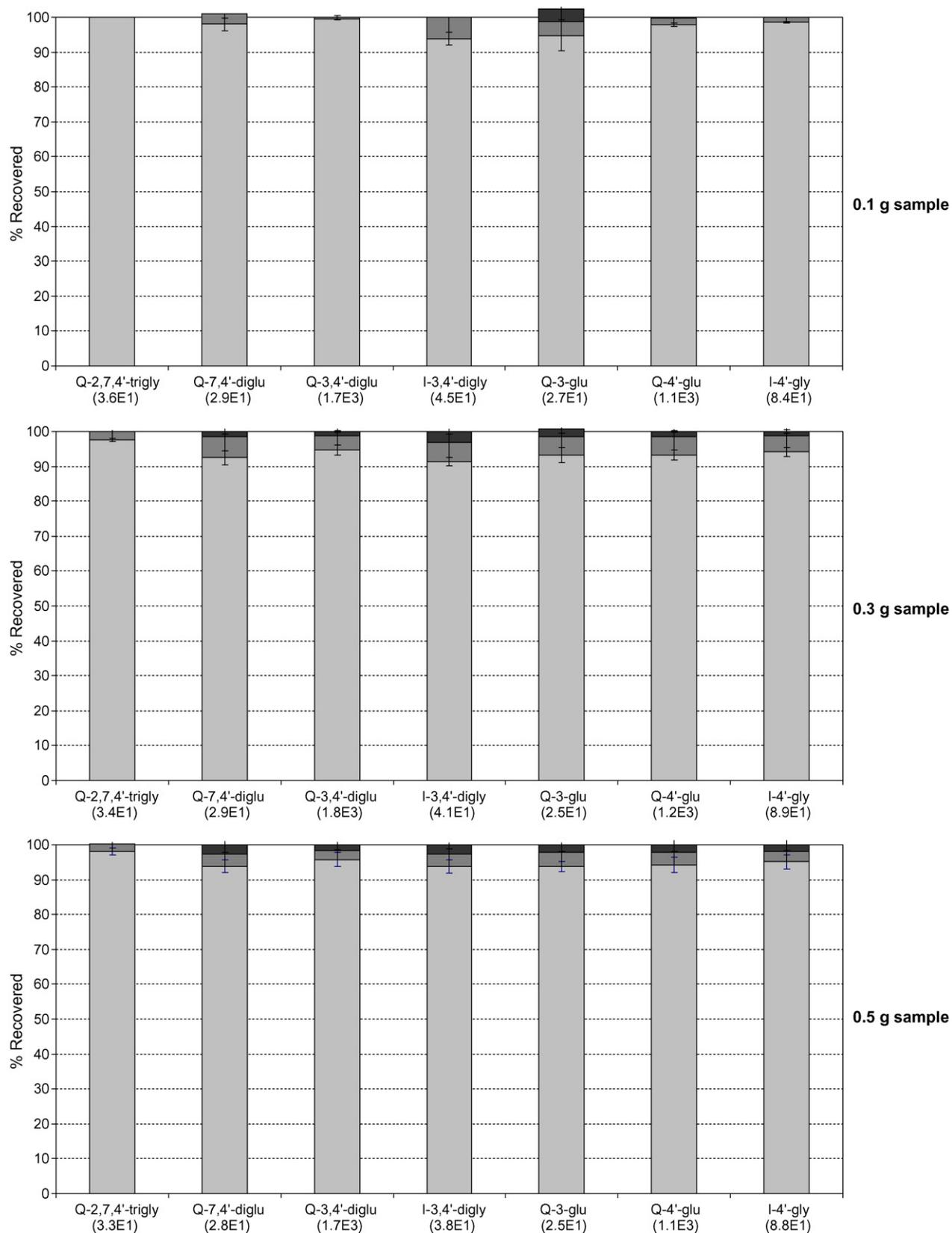
**Fig. 4.** Effect of sample weight on recovery in the three collected extracts (pressurised liquid extraction). (■) 1st extract; (■) 2nd extract and (■) 3rd extract. The total recovery in all three extracts ( $\mu\text{g}$  quercetin-equivalents/g dry weight) is shown in parenthesis below each compound. The error bars describe the standard deviation ( $n=3$ ).
