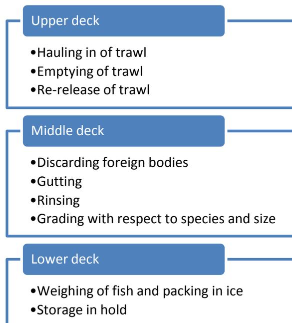
Figure 4.2. Catch handling process steps onboard Fishing vessel 1.
