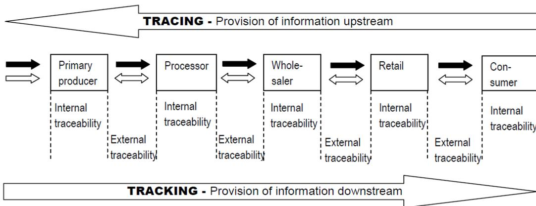
Figure 2.2. Illustration of traceability concepts in a food supply chain (Randrup *et al.*, 2008). Filled arrows show the product flow; open arrows show the information flow.
