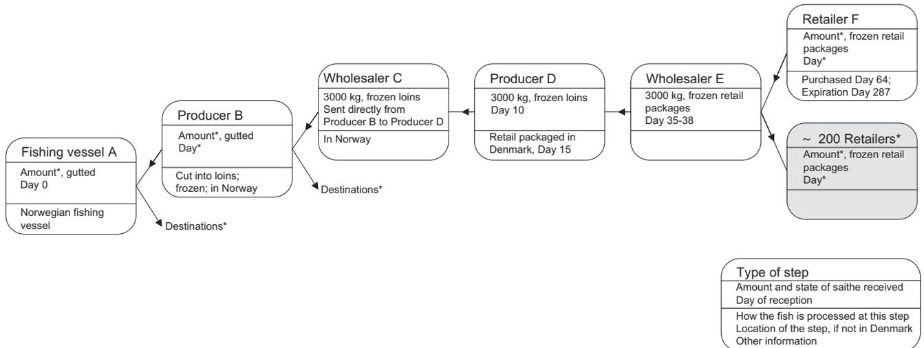
**Fig. 4.** Distribution network of Case 3: saithe. Arrows pointing left indicate tracing back (white boxes). Arrows pointing right indicate tracking forward (shaded boxes). Product flow is from left to right. \* = Unidentified for the researchers.
