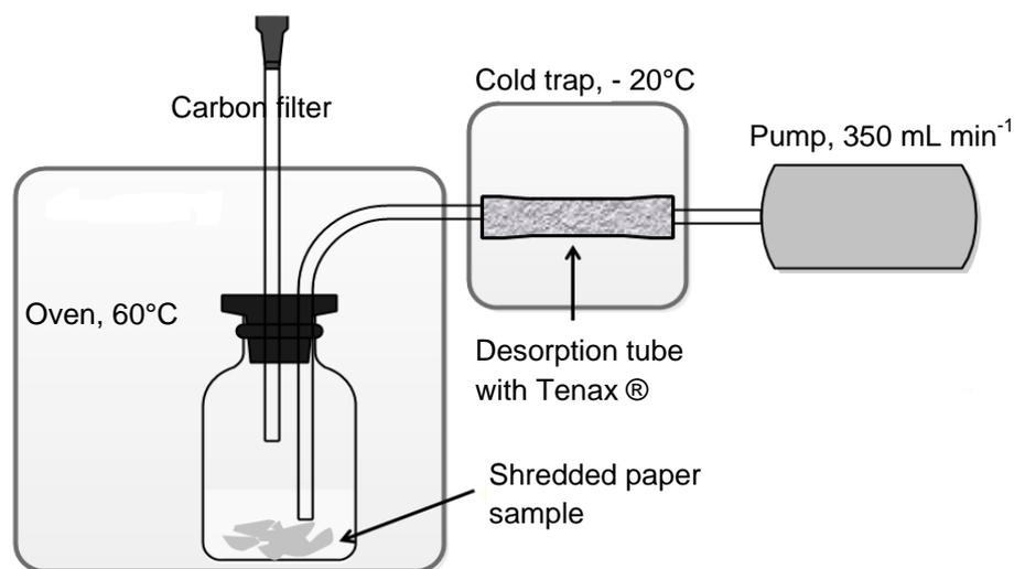
Figure 10. Set-up used for the purge-and-trap of VOCs from paper and board.
