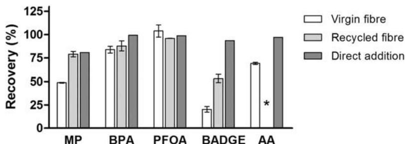
Figure 2. Recovery of 50 ng surrogates ( $\text{dm}^{-2}$ )<sup>-1</sup> in fortified paper samples after extraction. The direct addition is used as a control sample. Recovery for BADGE is calculated from undiluted sample. Standard deviation is indicated as error bars. \*The recycled fibre contained too high concentrations of the additive AA to be quantified.
