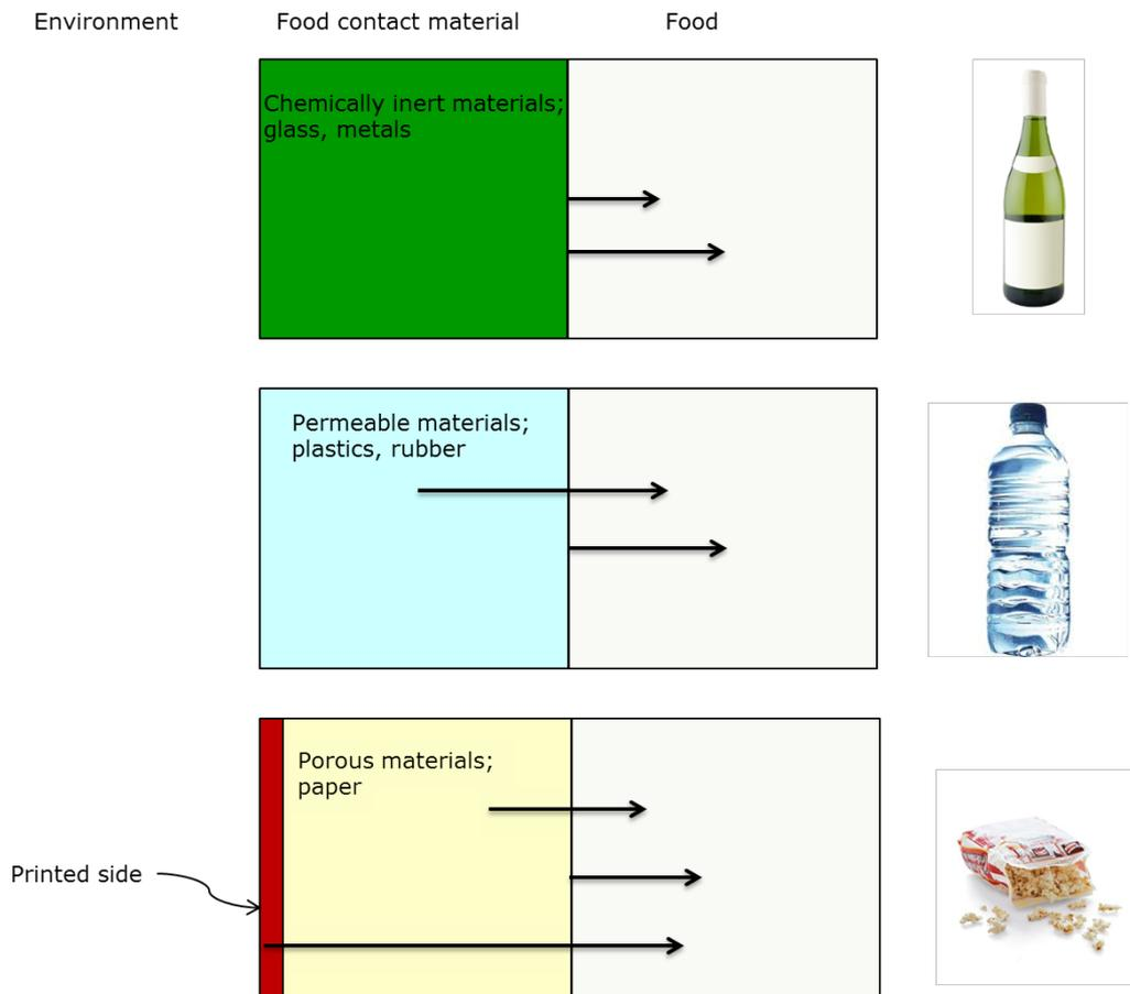
Figure 9. Migration processes for different packaging materials; glass or metal, plastic and paper. Porous materials such as paper and board offer almost no resistance towards mass transfer, allowing substances to migrate all the way through the material. Adapted from Barnes et al., 2007.
