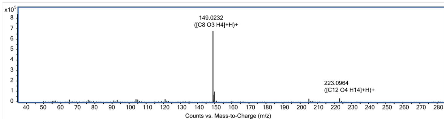
Figure 20. Fragmentation pattern of DBP in a) alkaline fraction 6 from sample S8 in obtained by UHPLC-ES+I-qTOF MS (at 100 V in collision energy, thus only in source fragmentation). b) Standard (5  $\mu\text{g}/\text{mL}$ ) with DBP and c) alkaline fraction 6 from sample S8 in obtained by GC-qTOF. In both cases, the fractions were diluted 1:1000  $v/v$  with ethanol.
