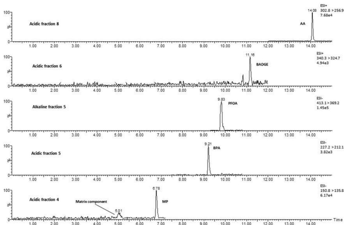
Figure 3. Illustrative chromatograms of the five surrogates in fractions from fortified virgin fibre. The fractions were diluted 1:10 v/v, except for acidic fraction number 6 with BADGE. The large peak of a matrix component in the MP chromatogram is clearly smaller in the fraction compared with the corresponding raw extract.
