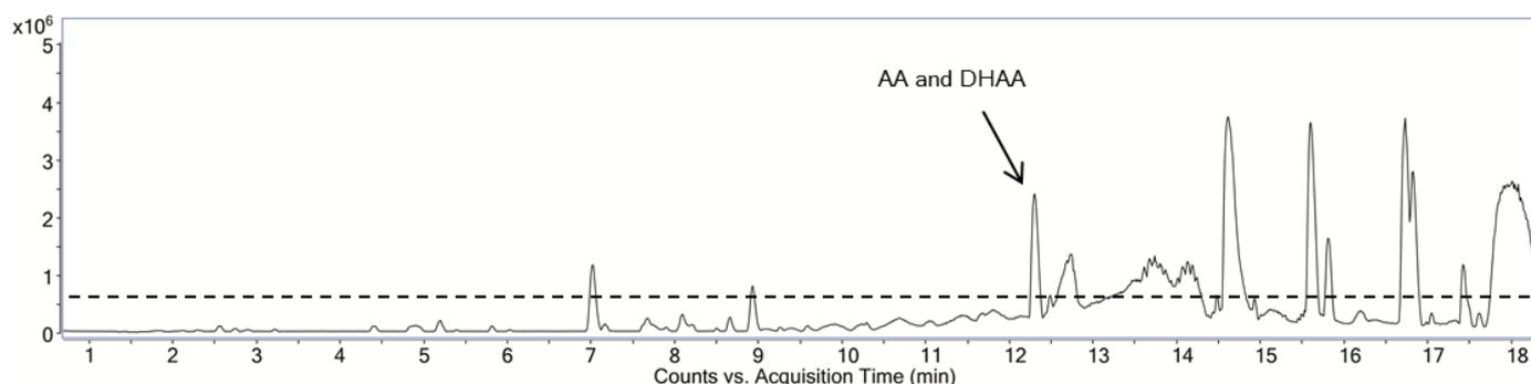
Figure 19. Base peak chromatogram (BPC) of alkaline fraction 8 from S4 acquired by UPLC-ESI+qTOF MS. This fraction had a toxicological response in the AR assay. The co-eluting DHAA and AA, two of the compounds selected for further analysis are indicated in the BPC. The dotted line represents the cut-off.
