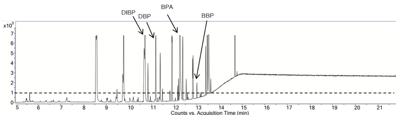
Figure 18. Base peak chromatogram (BPC) of acidic fraction 6 from sample S8 acquired by GC-qTOF. This fraction had a toxicological response in the ER assay. The four compounds; BPA, DBP, DIBP and BBP, selected for further testing are indicated by arrows in the chromatogram. The dotted line represents the cut-off.
