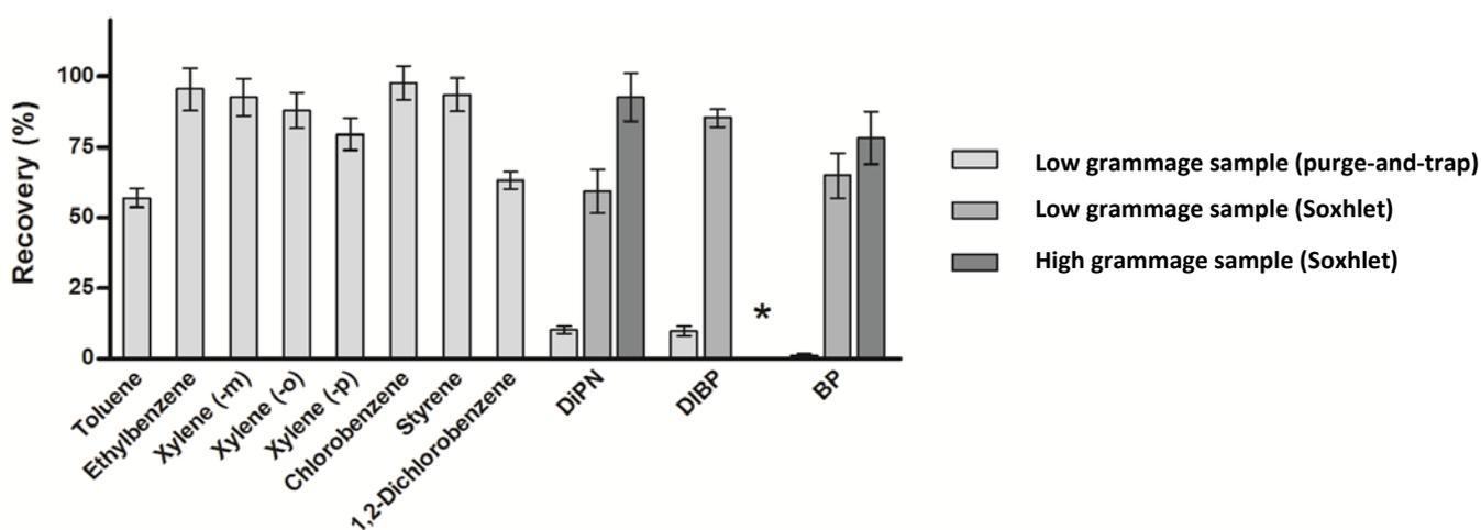
Figure 13. Recoveries of  $167 \text{ ng surrogates dm}^{-2}$  in fortified virgin fibre after purge-and-trap as well as after Soxhlet extraction and in fortified recycled fibre after Soxhlet extraction. Standard deviation is indicated as error bars. The surrogates are arranged from left to right according to their boiling point. \*The recycled fibre contained too high concentrations of DIBP after the Soxhlet extraction to be quantified.
