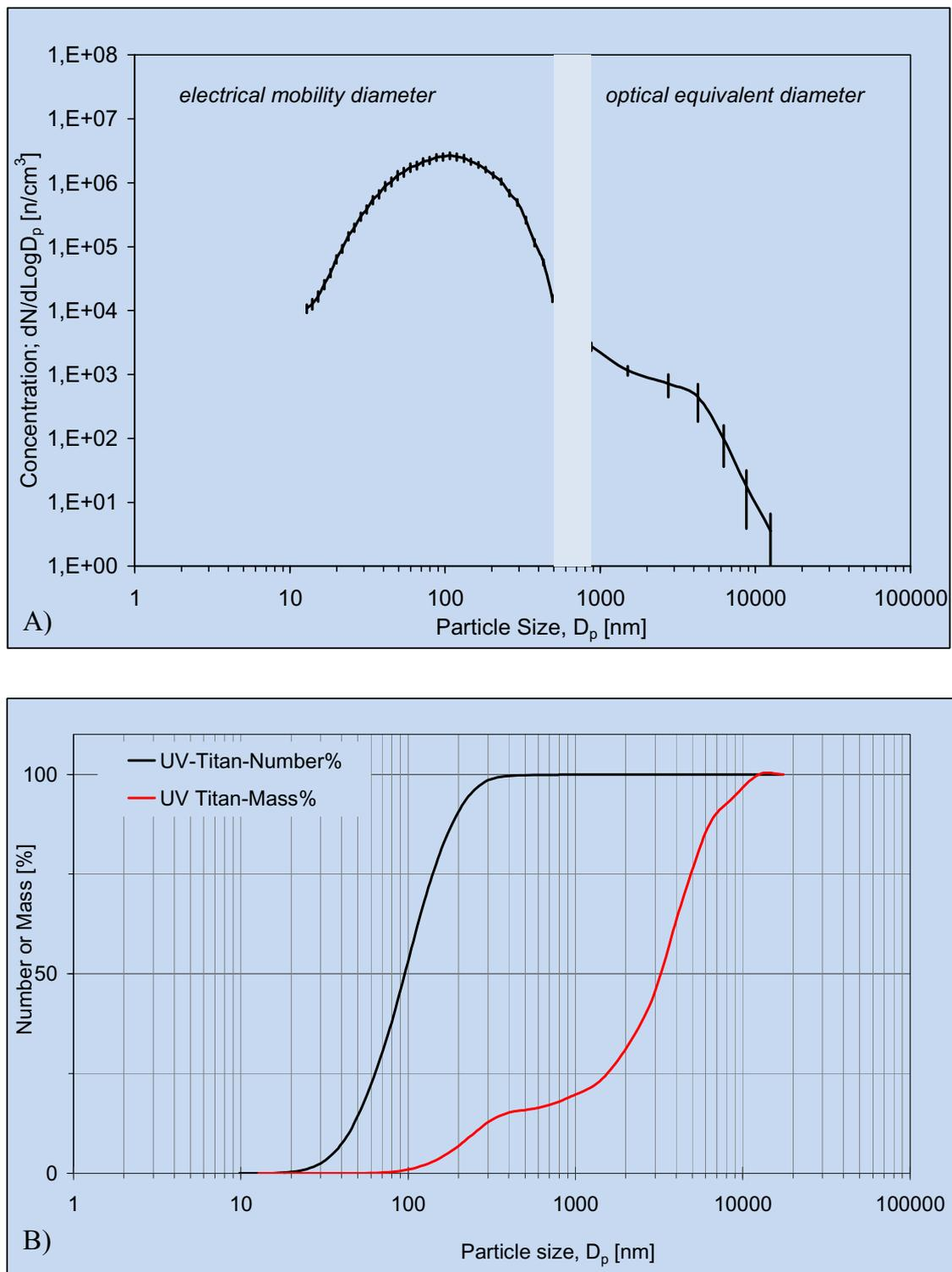
**Figure 2 Characteristics of the exposure atmosphere.** A) Particle number size distribution of the UV-Titan L181 in the exposure chamber. Data are based on nine one-hour exposure measurements. Mean  $\pm$  SD. B) Accumulated number and mass concentration of particle concentrations in the exposure chamber. It is assumed that the optical and mobility particle sizes can be directly compared and data gap is filled by linear interpolation.
