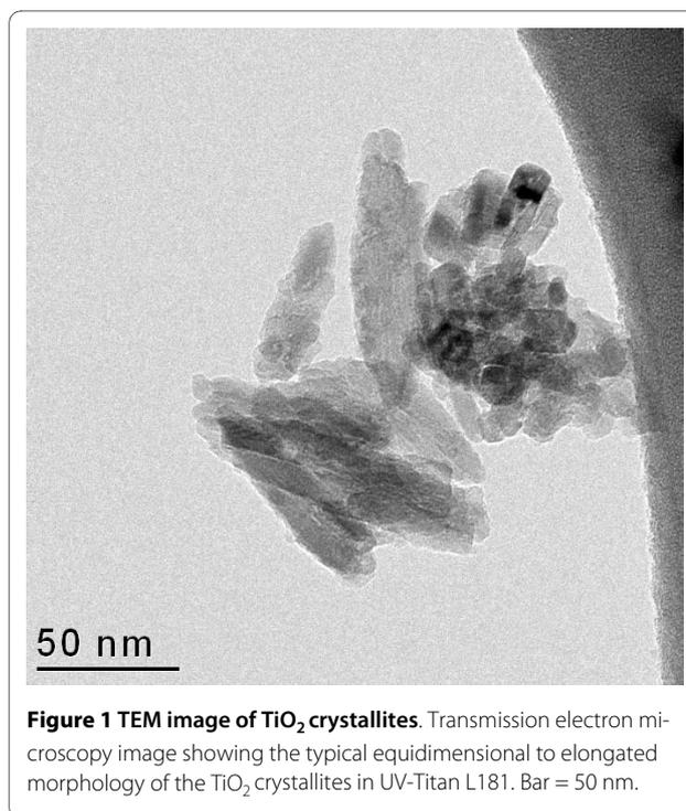
**Figure 1 TEM image of TiO<sub>2</sub> crystallites.** Transmission electron microscopy image showing the typical equidimensional to elongated morphology of the TiO<sub>2</sub> crystallites in UV-Titan L181. Bar = 50 nm.
